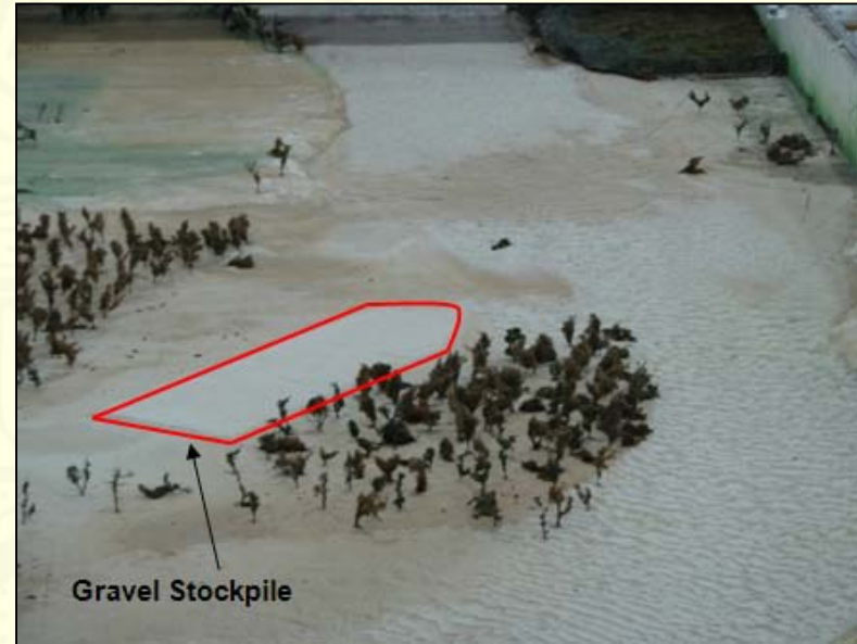
Constructed model Gravel Stockpile
