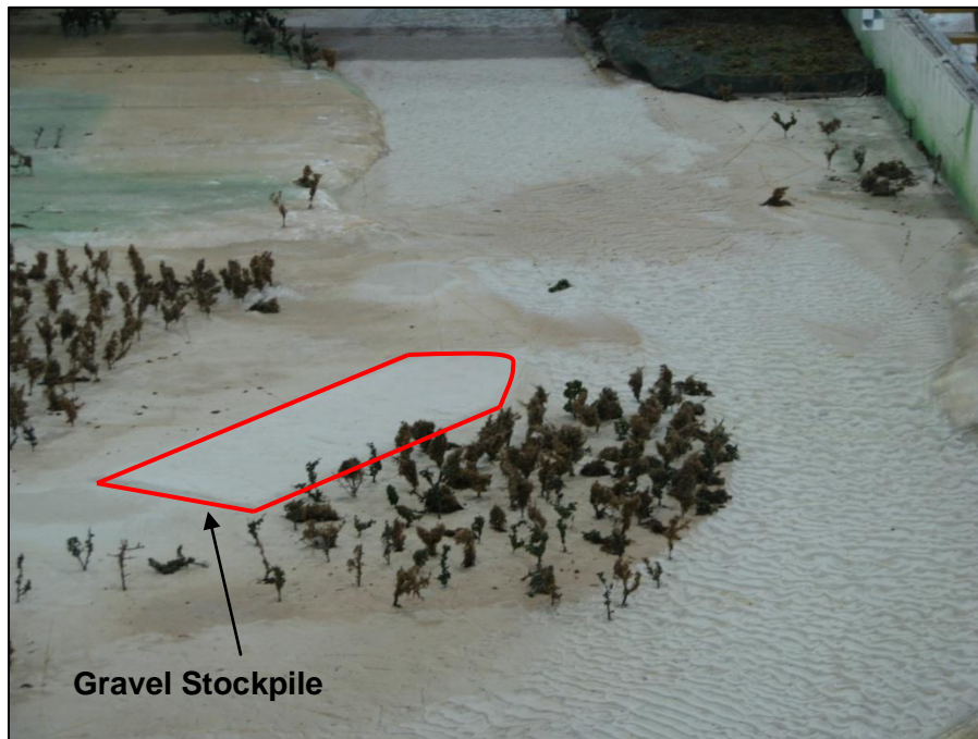
Figure 2-10: Constructed gravel stockpile after 145,000-cfs testing.
