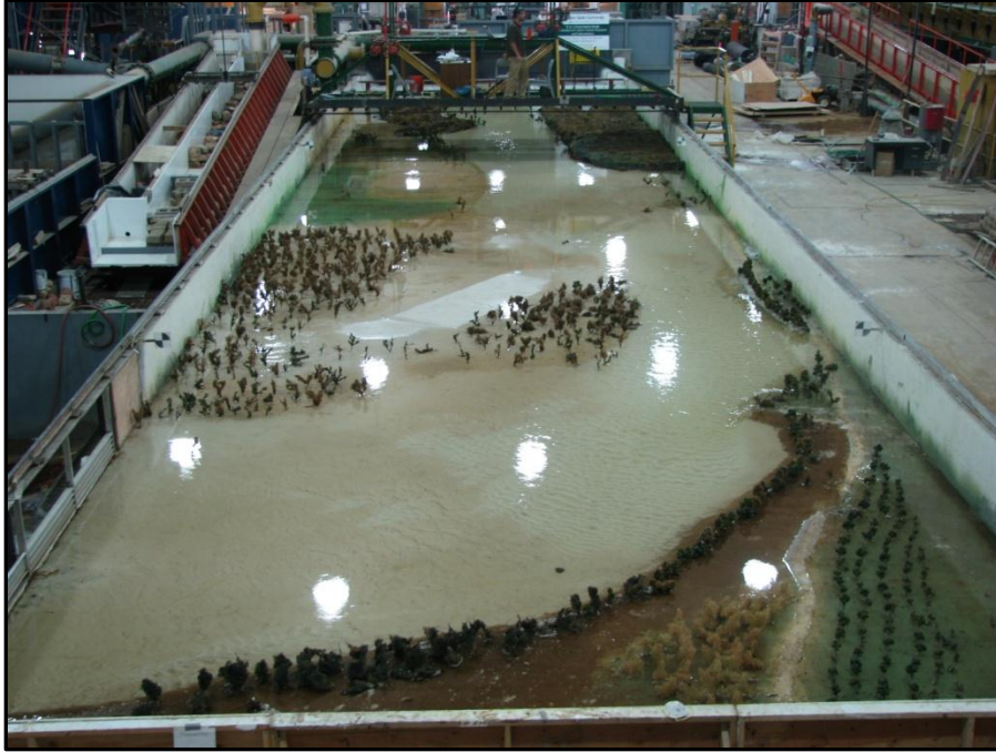
Figure 3-8: 145,000-cfs Gravel-stockpile configuration testing.
