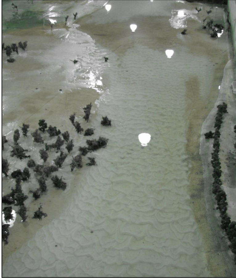
Figure 4-9: Ripple formation during 145,000-cfs Baseline testing.
